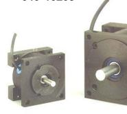
The MPC is a power-off brake module with an output shaft. It is designed for use as a coupler between C-Face motor and a C-Face gear reducer. Never mount a pulley or sprocket onto the brake output shaft as the MPC will not accomodate any type of overhung load applications.
