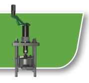
The Svendborg Brakes Anti-Glazing Groove tool leverages expertise in mitigating yaw brake noise. By cutting a specially-shaped groove into the brake disc it is possible to remove existing glazing and prevent it from occurring in the future. The groove tool helps to remove the build-up of powdered material.
