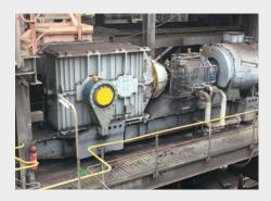
**Problem:** A major energy company in Australia needed reliable replacement lowspeed backstops (LSBs) for use on six incline conveyors that move coal out of a mine to an adjacent power station. The existing LSBs were being removed every two years for inspection and often needed to be replaced due to premature failure.
