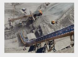
**Problem:** Most accidents on mining conveyors are caused by the stored energy in the belt. If not properly protected, a loss of power at a mine can allow loaded inclined conveyors to reverse direction, causing damage to expensive equipment. Reverse rotation of conveyor belts can be prevented by installing a standard backstop or a torque-limiting backstop. However, to allow the crew a safe maintenance routine, a loaded conveyor belt needs to be slowly rotated backwards to clear the belt.
