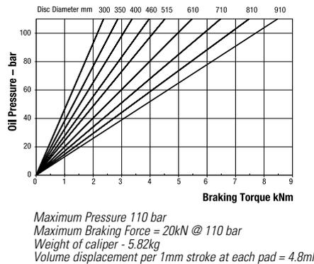
Normally one or two calipers are used per disc, but the number may be increased depending on disc size. The brakes may be positioned at any angle around the periphery of the disc. A range of brake discs is available from Twiflex (see Disc and Hub Assemblies).
