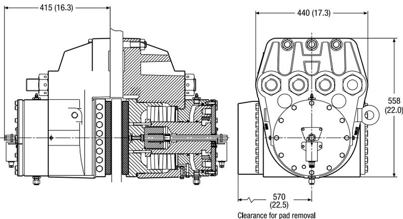
The Twiflex VMS2 disc brake caliper is comprised of two modules bolted to a central mounting plate, 12mm thicker than the brake disc. Minimum disc thickness is 38mm and minimum disc diameter is 1500mm with no maximum except for practical limitations.
