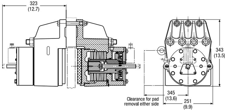
The Twiflex VKSD disc brake caliper is comprised of two halves, or spring modules, and is suitable for use with a minimum disc thickness of 20mm. The modules are mounted each side of a central mounting plate 12mm thicker than the brake disc. Minimum disc diameter is 1000mm.
