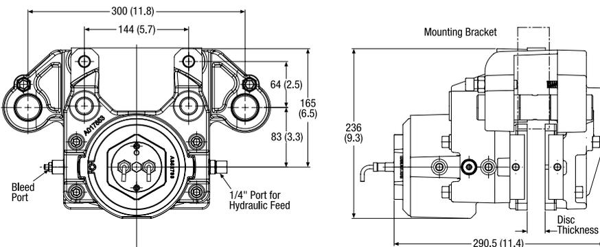
The Twiflex VCS-FL disc brake caliper comprises a single spring module forming the 'active' side of this floating unit and is available for use where space is limited or to accommodate axial disc float of  $\pm 6$ mm.
