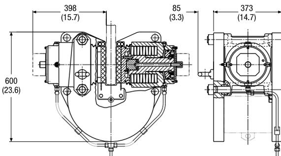
The Twiflex VS Mk2 disc brake caliper is comprised of two modules secured between U-shaped top and bottom mounting plates by tie rods.
