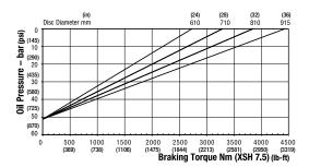
Maximum Braking Force XSH 7.5: 11.2kN (2517.86 lbf) Minimum Pressure for full retraction: 63 bar (914 psi) Weight of caliper and thruster - 13.62kg (30.03 lb) Weight of thruster only - 4.4kg (9.70 lb) Volume displacement of thruster at 6mm (0.24 in) retraction = 9.1ml (0.30 fl oz)
