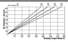
Maximum Pressure 7 bar (102 psi) Maximum Braking Force = 1.9kN @ 7 bar (427.14 @ 102 psi) Weight of caliper and thruster - 9.52kg (20.99 lb)
