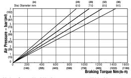
Maximum Pressure 7 bar (102 psi) Maximum Braking Force = 3.6kN @ 7 bar (809.31 @ 102 psi) Weight of caliper and thruster - 10.37kg (22.86 lb)
