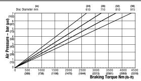
Maximum Pressure 7 bar (102 psi) Maximum Braking Force = 11kN @ 7 bar (2472.89 @ 102 psi) Weight of caliper and thruster - 11.28kg (24.87 lb) Weight of thruster only - 2.06kg (4.54 lb) Volume displacement of thruster at full stroke = 426ml (14.40 fl oz)
