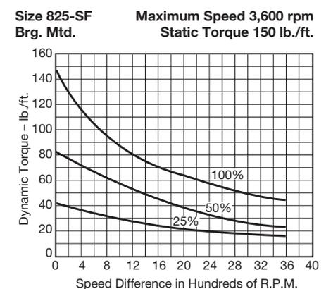
NOTE: Torque values are in inch lbs. for size 400 and smaller, and in ft.lbs. for size 500 and larger.
