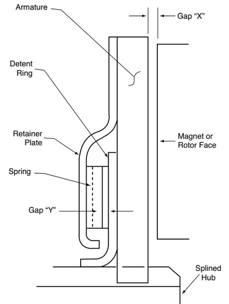
This can happen with excess vibration or mishandling. To reset the autogap, move the armature assembly toward the magnet or rotor. This can be done by 1) or 2) below:
