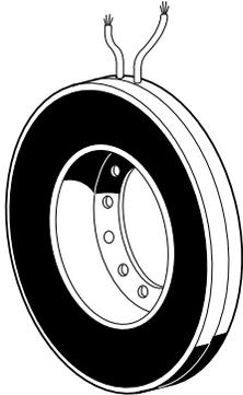
Since LK has a lower coefficient of friction, lower torque capability results. With LK facing, static torque capacity is only about 60% of catalog rating for any given size. So if a specific size clutch or brake is chosen for its rated torque capacity and LK facings are substituted for standard, a larger size unit will be needed to provide the same torque.
