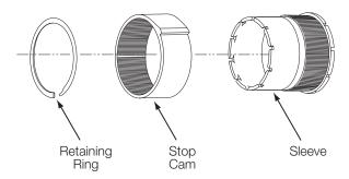
To adjust the stop collar output orientation:
