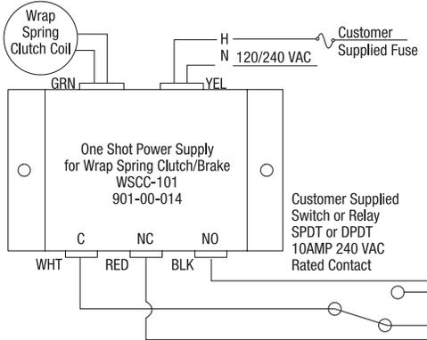
Actuating the single pole, double throw (SPDT) switch energizes the solenoid coil. Releasing or resetting the switch charges an internal capacitor. A minimum of 20 milliseconds cycle time is required between operations.
