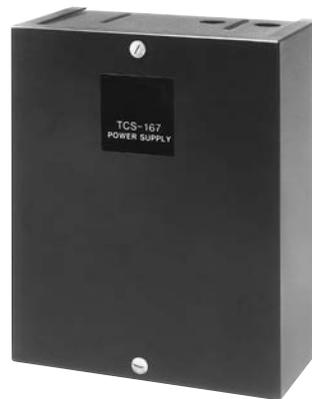
The TCS-167 power supply is designed to provide the correct power input to TCS-210 and TCS-220 tension controls. Its switch selectable input allows the user to adapt to 120 or 240 VAC. It has dual voltage circuits to provide low voltage power and anti-residual output as well as power to operate a brake. The TCS-167 is available with an open frame for control panel mounting.
