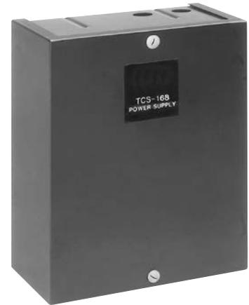
The TCS-168 power supply is designed to provide the correct power input to the TCS-310 Dancer Splicer Control. Its switch selectable input allows the user to adapt to 120 or 240 VAC. It has dual voltage circuits to provide low voltage power and anti-residual output as well as power to operate two brakes. The TCS-168 is available with an open frame for control panel mounting.
