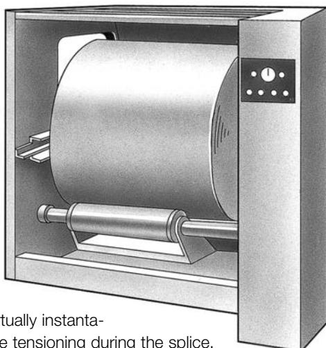
Tension variations of 25% or more may be possible during acceleration or deceleration, and 10% or more during running due to out of round rolls or variations in the process machines.
