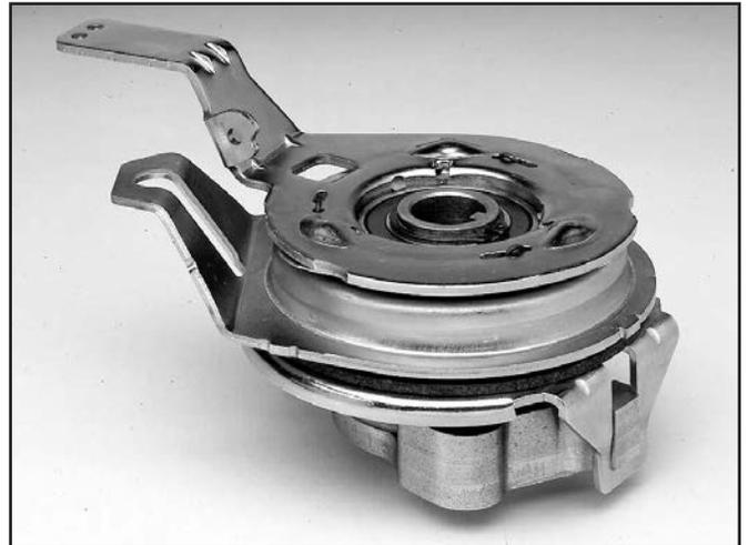
11. Reinstall the BBC mounting bolt. Torque the BBC mounting bolt to 48 ft-lbs. (65 N-m) for a 3/8-24 UNF or a M10 x 1.25-6g mounting bolt (contact Warner Electric personnel for assistance with other thread sizes).
