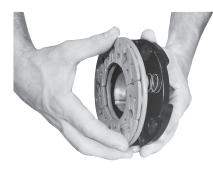
Straight springs must fit into grooves in armature hub.
