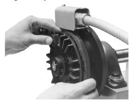
Attach the new friction material segments to the brake magnet or clutch rotor with the screws through the appropriate access holes. Apply one drop of Loctite<sup>®</sup> (grade AA or equivalent) to each screw.
