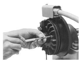
8. Insert the two new armature segments.
