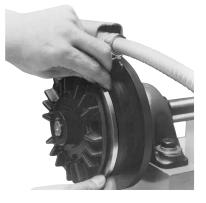
Attach the new armature segments to the cast iron carrier with hex head capscrews, lock washers and washers. Apply one drop of Loctite (grade AA or equivalent) to each screw. Tighten to the appropriate torque for your size unit.
