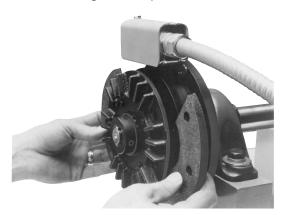
6. Insert two new friction material segments. The recessed holes should be facing away from the magnet body.
