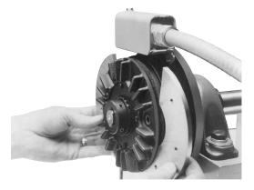
Remove the screws that attach the friction material segments to the brake magnet or clutch rotor through the appropriate access holes.
