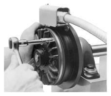
10. Reset the Autogap<sup>™</sup> by pressing the armature toward the magnet or rotor.
