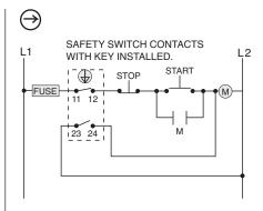
Special wiring for the safety-interlock switch to prevent tampering. The N.O contact 23-24 short circuits the coil of motor starter (M) with key removed. If the N.C. contact 11-12 were jumpered, the fuse would blow when the key is removed from the switch and an attempt is made to restart the circuit.
