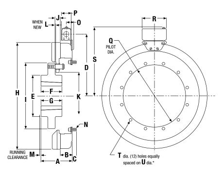
$<sup>^*\</sup>mbox{Mounting holes}$  are within .010'' (.254) of true position relative to pilot diameter.
