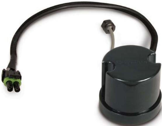
The PQS is a bi-directional current limit control. The control monitors current during actuator motion and quickly stops the actuator if an object gets in the way or at the end of stroke. The actuator will remain off until power is reapplied. The current limit setting is adjustable with two potentiometers that are accessible through two plugged holes on the side of the housing.
