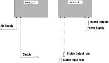
Above information is for basic control units and subject to change without notice. Double or triple clutch control units for two or three speed dredge pump drives with quill mounted clutches are also available. (9908-02 and 9908-03)
