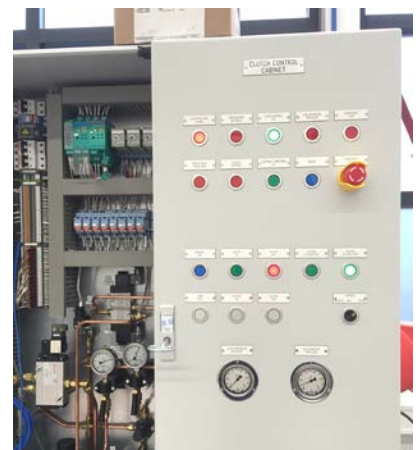
Typical Wichita clutch control cabinet and panel
