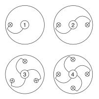
Number of Air Hose Connections: 1, 2, 3 or 4 depending on the application and unit size.
