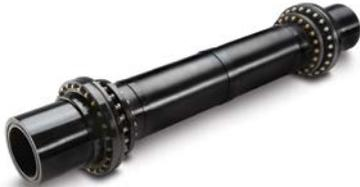
Unique diaphragm design permits high-torque density and low weight. Designed for years of dependable, low-maintenance performance. Multiple, separated, convoluted diaphragms in a pack, provide a built-in, fail-safe feature while allowing the greatest design flexibility for the most demanding applications. Units are API 671 compliant. Diaphragms are shot-peened for improved fatigue strength and stress corrosion resistance.
