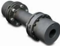
Specifically designed for the process pump and general industrial applications. Standard coupling is fully compliant with the requirements of API 610 / ISO 14691. Plug-in spacer design allows installation and removal without disturbing the hubs.
