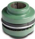
Sure-Flex couplings, a TB Wood's original, utilize a rubber (EPDM or Neoprene) or Hytrel™ thermoplastic flex element (sleeve) to transmit torque and accommodate shaft misalignments. Sure-Flex couplings have exceptional torsional flexibility, and the 4-way flexing action absorbs virtually all types of shock, vibration, misalignment, and end float.
