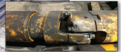
Damage due to bolts coming loose on competitor U-Joint
