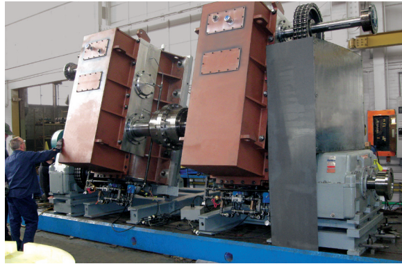
Photos show Nuttall's massive in-house custom-built test stand with two of the 15,000 lb. Fort Street bridge reducers mounted and being tested on a 75-degree incline per specification.
