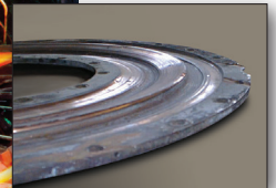
Severe damage on non-genuine copper wear plate
