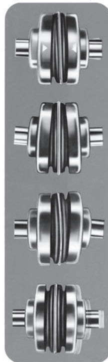
Four basic conditions of shaft misalignment or movement that determine selection of the correct coupling.
