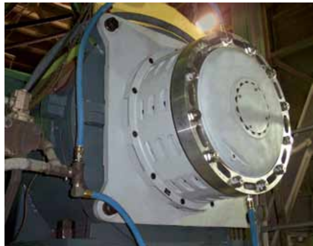
Industrial Clutch LKB brake on a dragline
