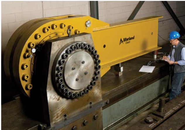
Massive Marland BC1200-MA low-speed holdbacks, with a torque rating of 1626000 Nm (1.2 million lb.ft.) are the largest conventional backstops ever built.
