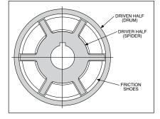
As the interior "spider" hub of a Centrifugal Clutch rotates, centrifugal force causes the shoes with friction facing to expand outward into the driven drum. The greater the rotational speed, the greater the centrifugal force and the greater the transmission of torque via the shoes from input hub to output drum.
