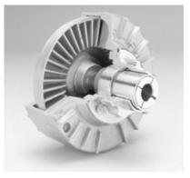
The fluid coupling is an enclosed system. The input portion goes into a vaned member called the "runner." The output part is similarly vaned and referred to as the "impeller." Between the two pieces is a volume of hydraulic fluid. As the runner begins to rotate it starts rotating the fluid. The fluid transfers that rotation to the impeller and from there to the output shaft of the coupling. As speed increases so does the torque transfer.
