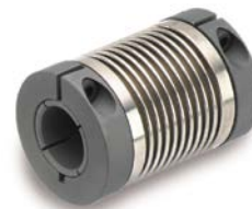
Flex Ni couplings provide rotation position integrity. This is achieved through high torsional stiffness while still accommodating large amounts of lateral and angular misalignment due to low spring rates in these directions.
