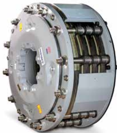
Air cooled, spring-set, air released AirMaKKs SSB high torque brakes by Wichita Clutch are designed to provide low speed braking assistance in applications including conveyors, cranes and drawworks where they serve as a main brake that provides both parking and e-stop braking functions. AirMaKKs brakes, featuring stainless steel torque plates, are also available for marine deck applications where sea spray and direct seawater splash are prevalent.
