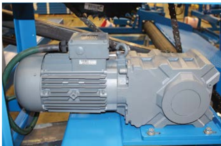
A Bauer BK Series geared motor drives a roller which rotates the large cable reel as it coils. The output shaft of the geared motor is coupled, via chain and sprocket, to the drive roller.
