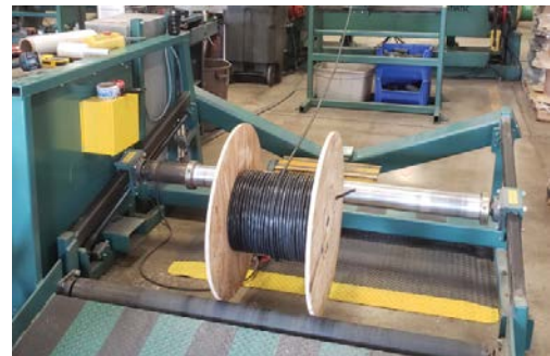
RD10 reels are “rim driven” allowing for quick change out and loading of large wire and cable spools.
