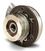
Warner Electric engineers developed a modified CMS (Commercial Mag Stop) clutch to meet a pump jack OEMs function and performance requirements. The clutch assembly mounts directly to the engine shaft and features a double-groove pulley to accommodate twin V-belts that drive the pump shaft.
