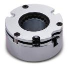
Matrix spring-applied, electromagneticallyreleased 1EB Series servo motor brakes are widely used on industrial robot applications. The brakes maintain torque during static/ holding operations and occasional E-stop (dynamic stopping) engagement in the case of power failure.
