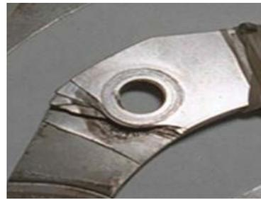
Figure 1: Blade failures where the disc material bent around the traditional round bushings.
