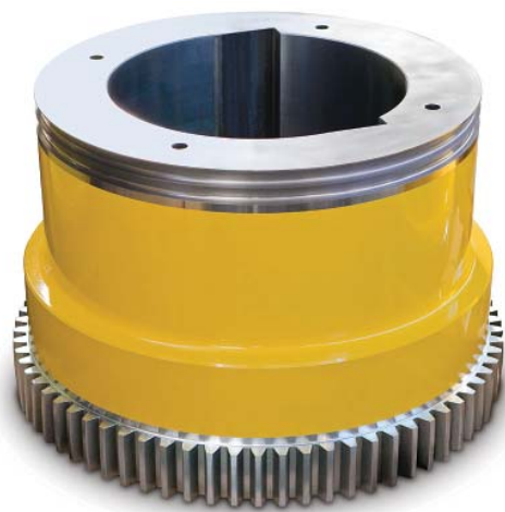
New Ameridrives replacement coupling featured crowned gear teeth and tangential keys and grooves cut into the bore to accommodate a customer-supplied seal
