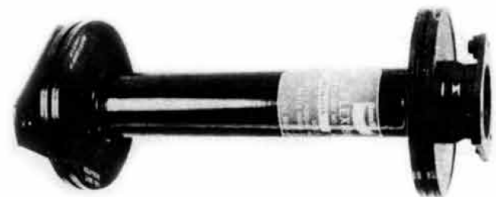
Contoured diaphragm coupling, 3900 In-lb @6,000 RPM, 2° misalignment with ± .100 inches axial travel.
