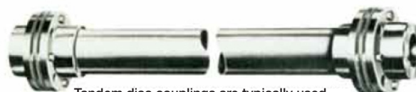
Tandem disc couplings are typically used on medium power pumps. The length is necessary to reduce angular misalignment of each disc pack from large amounts of offset seen by the equipment.
