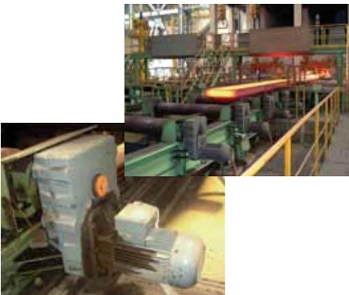
the standard solution for roller tables all over the world. However, no industry ever remains static and during the last few decades the demand for steel has continued to rise. This has put pressure on production plants to increase productivity. To facilitate increased throughput, plant engineers are specifying roller tables with ever increasing speeds; average speeds have risen from approximately 2m/sec to as much as 8m/sec.
