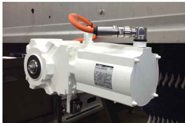
Bauer AsepticDrive PMSM models are designed for challenging washdown applications. The motors feature smooth surfaces and no cooling fins with corners or holes where bacteria can collect.
