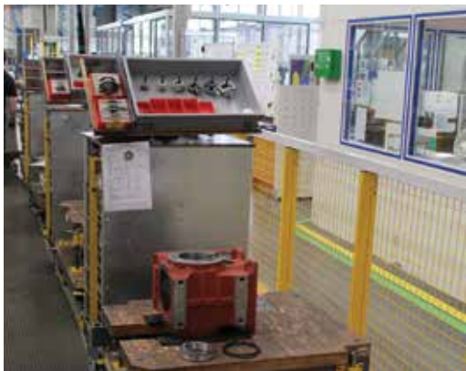
The production areas operate as one-piece-flow moving assembly lines.
