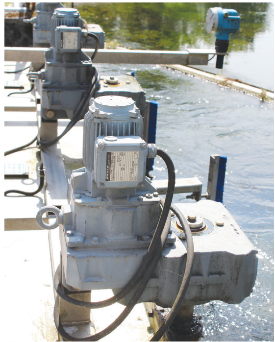
The Bauer gear motors provide compact, robust, and reliable operation, delivering the required low rotation speed.
