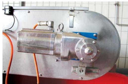
The stainless steel variant was introduced in areas where increased mechanical resilience was required.
