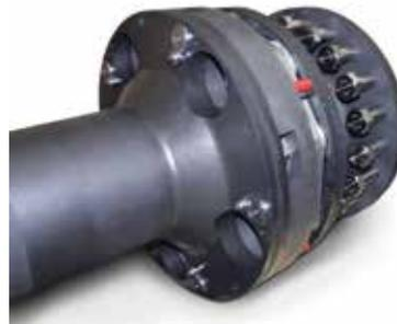
The low-speed coupling employs a set of shear pins that provide a simple, effective and precise method of disconnecting the drive system in the event of an overload.
