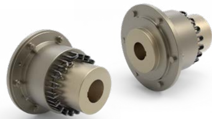
The coupling’s hub is manufactured from high quality materials, with the hub tooth profile scientifically designed to permit progressive loading under torsional shock conditions. The surface of the high tensile alloy steel grid spring is shot-peened to impede the propagation of cracks.
