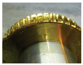
Figure 3: Worn gear teeth
