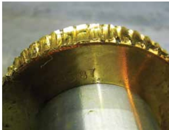
Figure 3: Worn gear teeth
