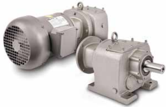
Boston Gear Series 2000 inline helical gear drives and gear motors require very low maintenance with unique rounded housing surfaces for easier cleaning, premium acrylic paint pigmented with 316 stainless steel flake for high corrosion and abrasion resistance, and integrated O-rings for high leak and ingress resistance. Other maintenance advantages include automatic entrapment of wear debris, large diameter oil fill/drain holes and synthetic lubrication.
