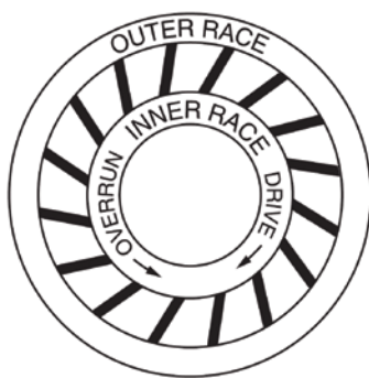
A sprag-type overrunning clutch generally consists of an inner race, an outer race, and a set of sprags evenly spaced in the annular space between them.
