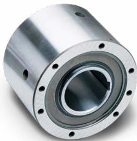
Model FSO 800 clutches have a torque capacity of 13,000 lb.ft. (17,680 Nm). Units are grease-lubricated with steel labyrinth seals and feature PCE sprags with Formchrome® and Formsprag “Free-action” retainers.
