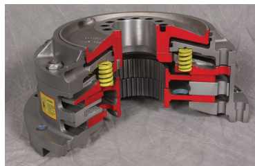
A disc brake is designed with rotating discs that are splined to a hub which is keyed or splined to the rotating motor shaft. These discs, or plates, slide axially when engaged and carry the friction lining. The braking surfaces are radial and the friction surface is defined by its outside and inside diameters. These discs engage the stationary components when actuated.
