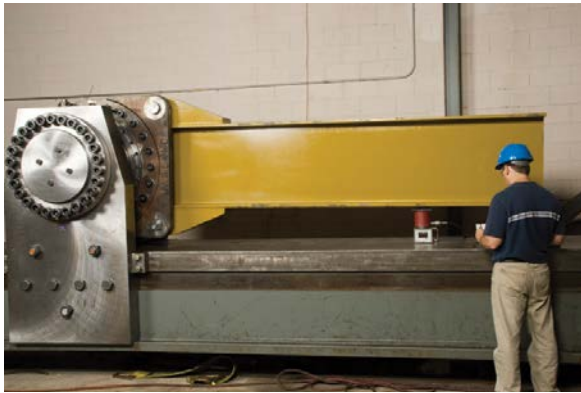
Marland Clutch senior product engineer Dave Divero does full torque load testing on a Marland backstop BC-375MA.
