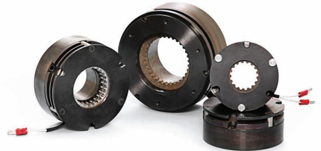
Brake coils require a DC voltage, which is normally provided by rectifying the AC voltage used to power the motor. Ensure that the DC voltage and current is always supplied to the brake coil while the motor is running, in order to keep the brake disengaged — as the speed of a servomotor can be controlled by varying the supply voltage.
